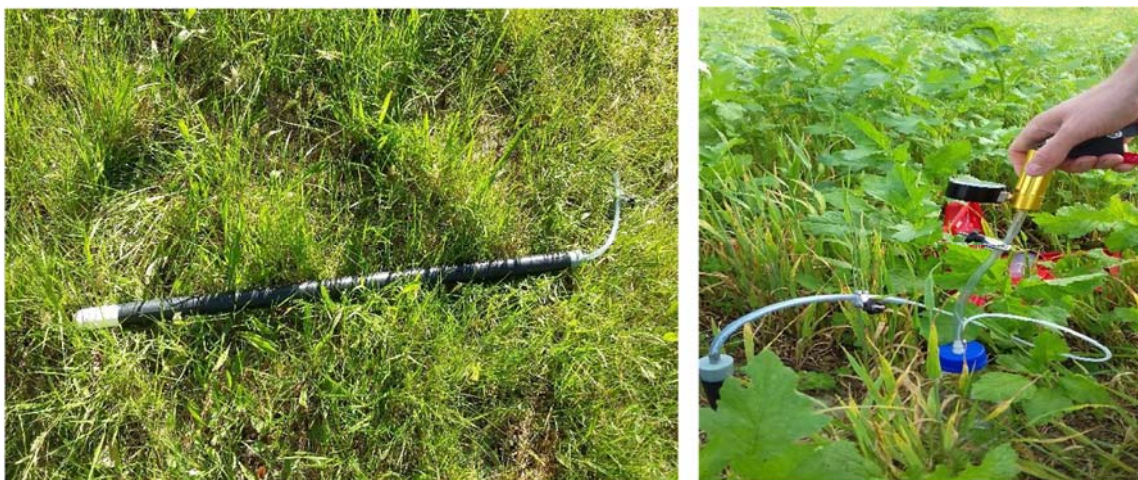
Figures 3.3 and 3.4. One of the porous pots used in the study and the vacuum pump apparatus used to extract the water sample. Each porous pot is approximately 1 meter long with the white, ceramic bulb being approximately 10 cm long.
